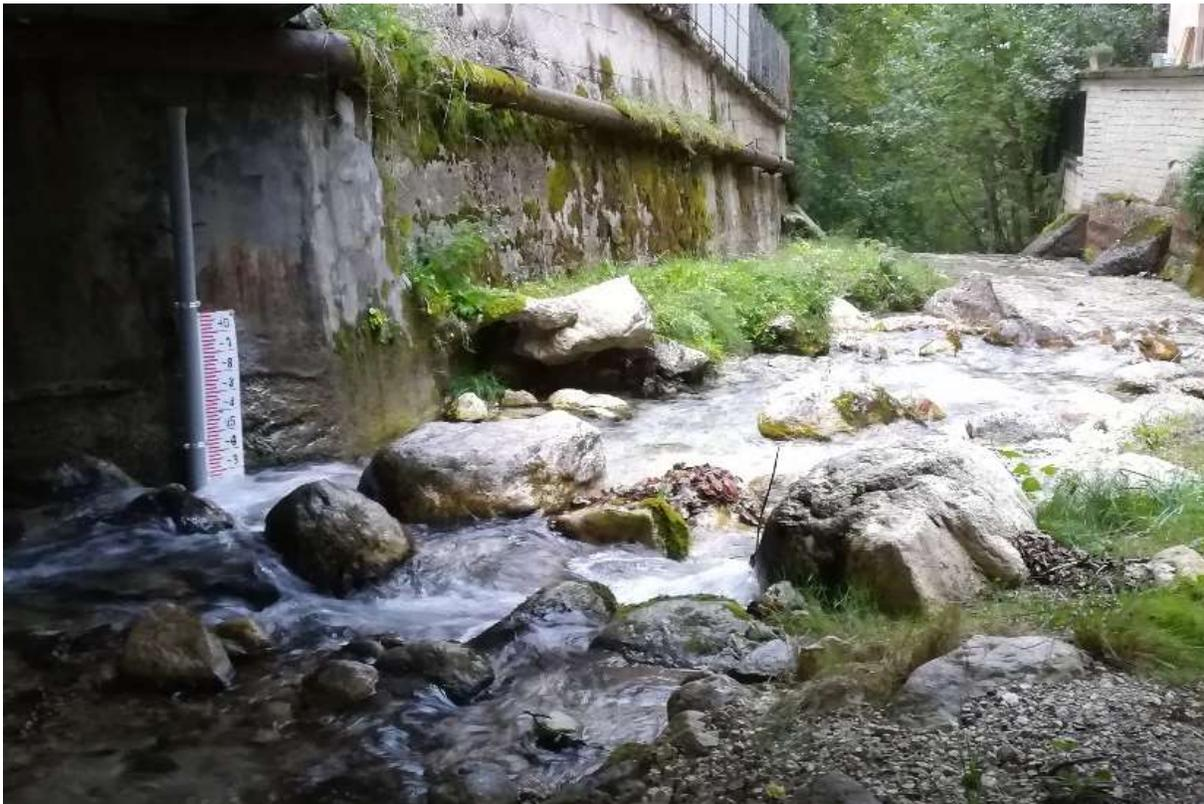
Figure 2.5. MA1 hydrometric gauge.
