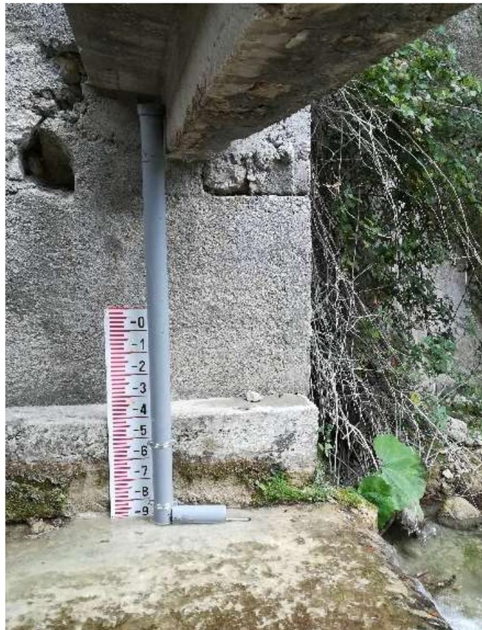
Figure 2.9. TA2 hydrometric gauge.
