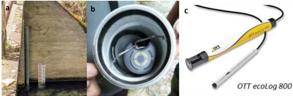
Figure 2.3. a) Hydrometric gauge; b) and c) OTT ecoLog 800 multiparametric probe, for continuous acquisition and remote transmission of data, including level, temperature, and electrical conductivity.
