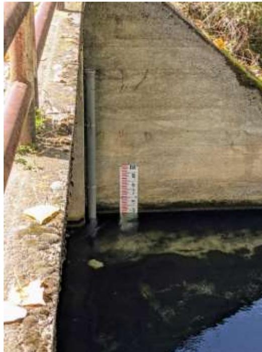
Figure 2.11. TI1 hydrometric gauge.
