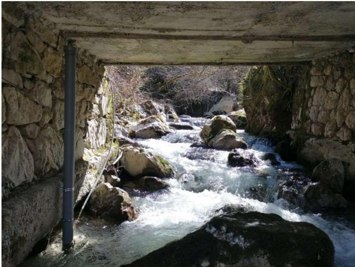
Figure 2.7. RU1 hydrometric gauge.
