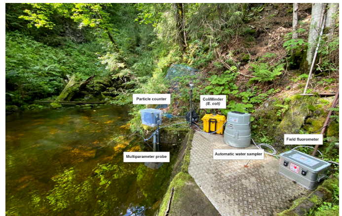
Particle counter, ColiMinder (encymatic activity analyser of E. coli ) and field fluorometer were installed at Sägebach spring, Austria, in order to detect contamination events (Photo: Simon Frank).
