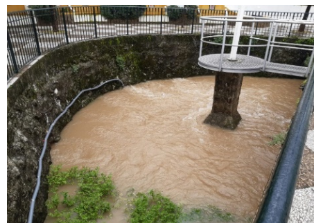
Figure 1: Algarrobal spring at Ubrique test site during a contamination event with high turbidity.
